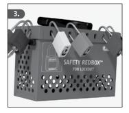
3. Close the cover. Make sure that it locks into place. Each employee involved in the maintenance then hangs his own personal padlock in one of the openings provided for this purpose in the cover and locks it. All enclosed keys are now securely locked until the last employee involved in the maintenance removes his personal padlock again.
