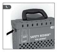
1. Open the cover using the push button on the left side.
